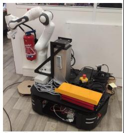
Fig. 1: illustration of mobile-manipulator collaborative robot
