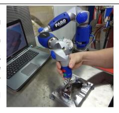
The goal of this project is to design and produce a measuring arm made up of 6 axes with 6 encoders to recreate a point cloud coming from a sensor at the end of the arm.
