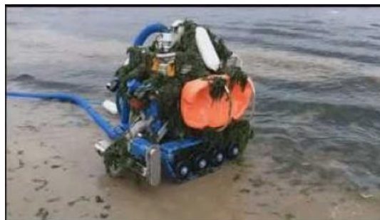
Figure 1: Underwater robot used for cleaning seabed
